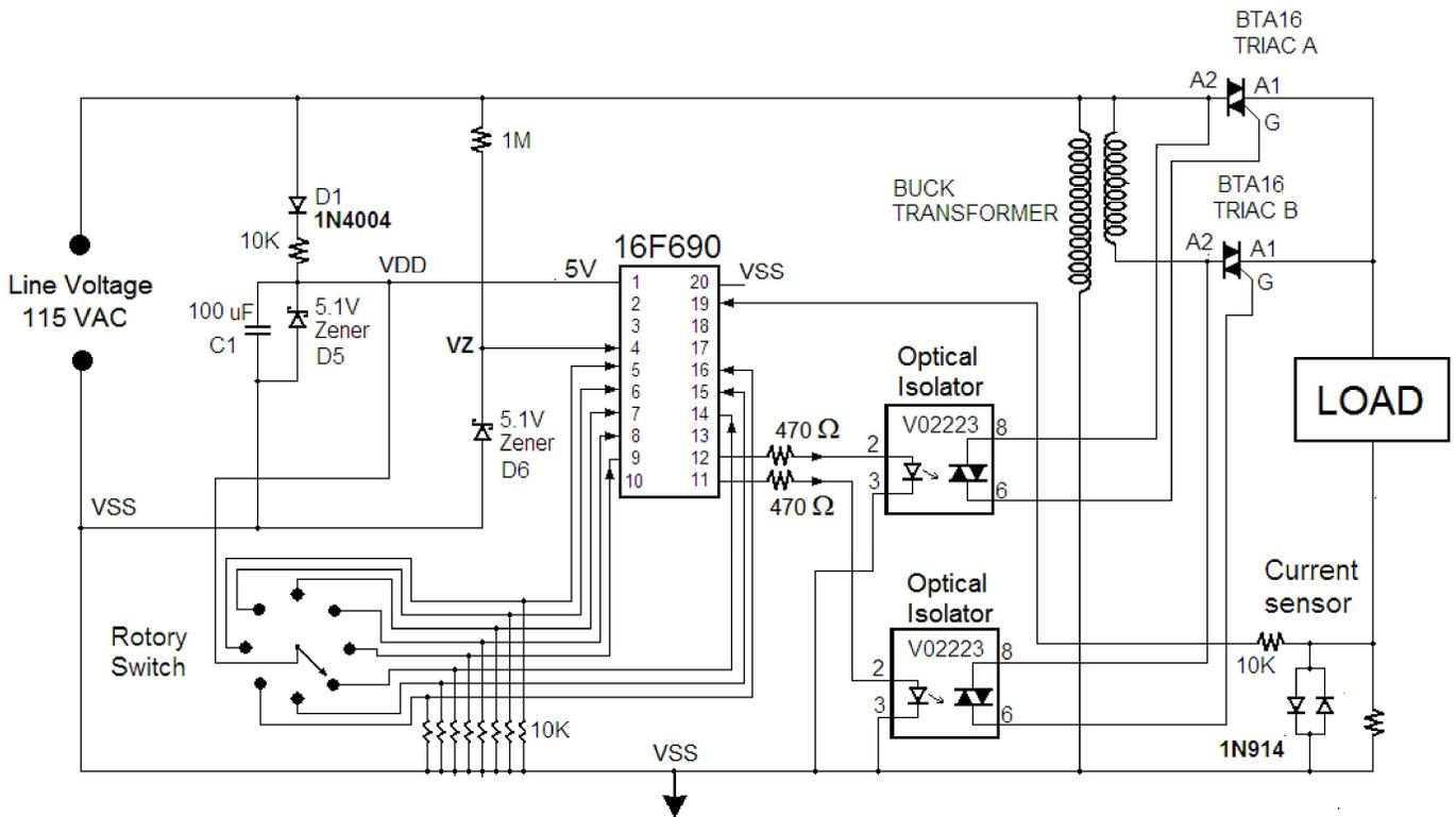
Figure 5 The 16F690 PIC microcontroller receives input from an 8 position rotary switch. Each position represents a desired power level. The controller determines the distribution of power levels needed to achieve the desired power. Optical isolators protect the microcontroller from the high load voltages and produce the signals required to trigger the switching triacs.
