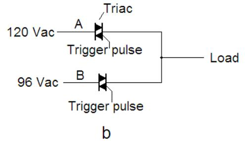
Figure 4 The single pole double throw switch, SPDT, used to regulate power is shown. In Figure 4 b the switch is implemented using two triacs.
