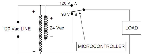
Figure 1 A microcontroller determines the timing of the Transcycle switch.
