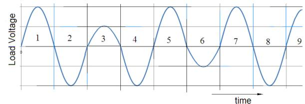
Figure 2 The load voltage is periodically reduced in half cycle increments. The voltage is shown reduced during the third and sixth half cycles.
