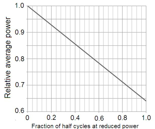
Figure 3 Reducing the load voltage in half cycle increments results in a reduced average load power. When none of the half cycles are at reduced power, the load power is 100%. When all of the half cycles are at reduced power the load power is at 64%
