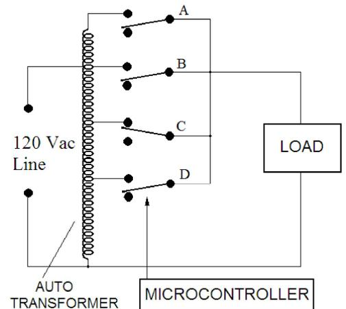
Figure 7 In this implementation power levels are switched between a number of levels provided by an auto transformer. One switch conducts at a time. Switch C is shown conducting. This results in a load voltage that is less than 120 Volts.
